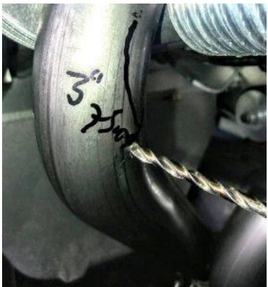
1. Mark and drill at 75mm (3") from Exhaust manifold
