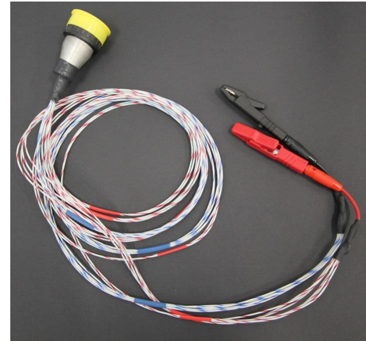
Troubleshooting wiring loom T080003
