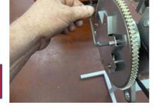
**6.** Reassemble the alternator ring gear and alternator fan with the cap screws and NordLock washers.
